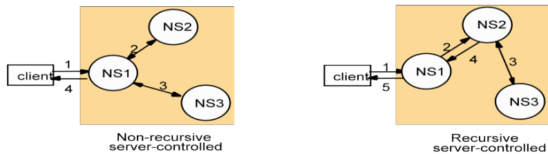
A name server NS1 communicates with other name servers on behalf of a client
